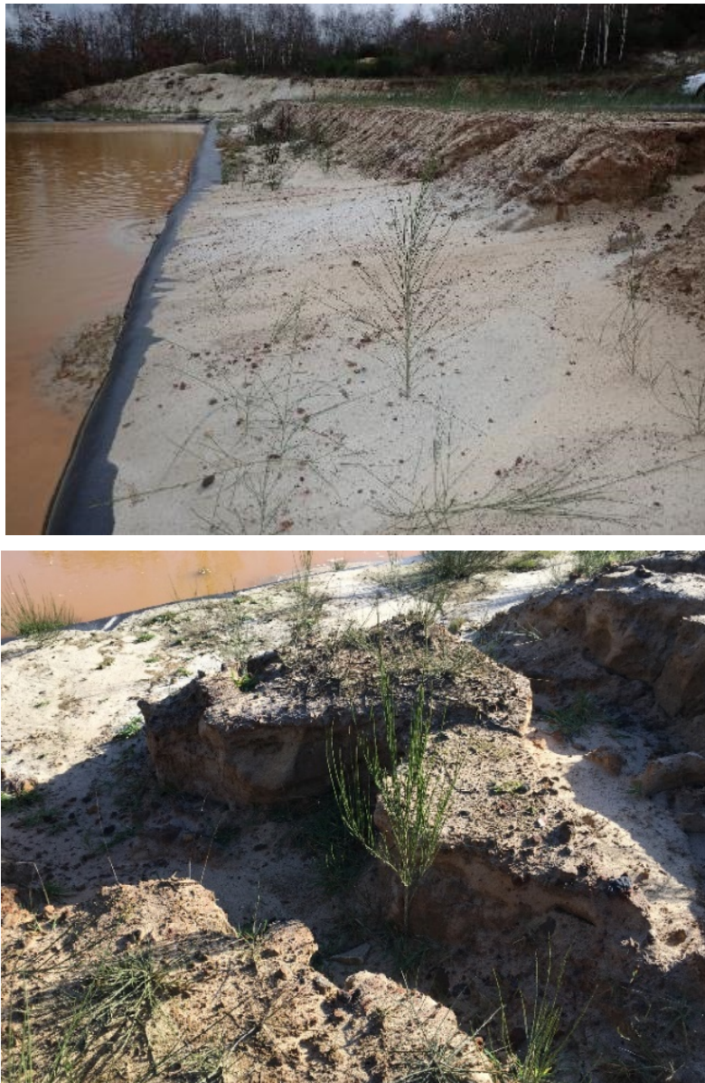
Figure 6 Intensive erosion of tailings in case study 2
